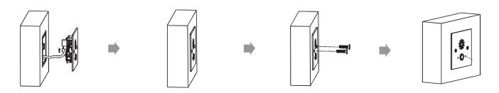
The device should be installed on the wall with 86 embedded box.
